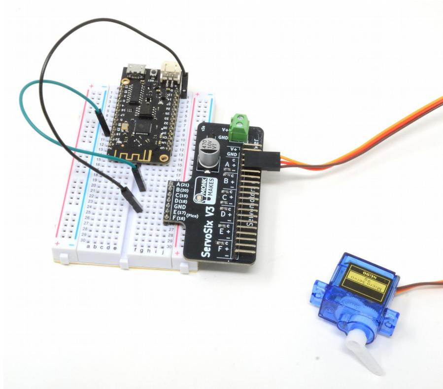
You will need to also provide power to the ServoSix using a battery box or connection from the microcontroller board.
