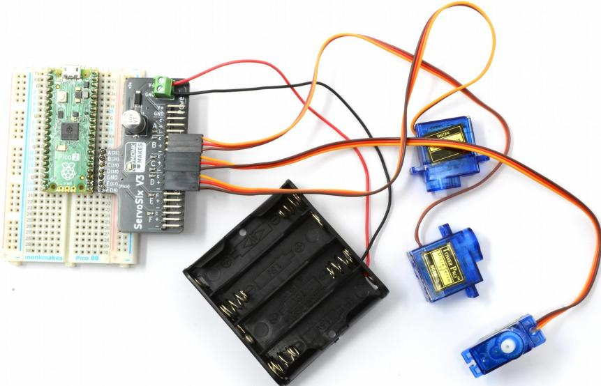
To use a battery box, such as the one shown above, first make sure that you choose one that supplies a voltage in the allowed range for your servomotors. Many servomotors will work quite happily at 6V, in which case a 4xAA battery box is ideal.
