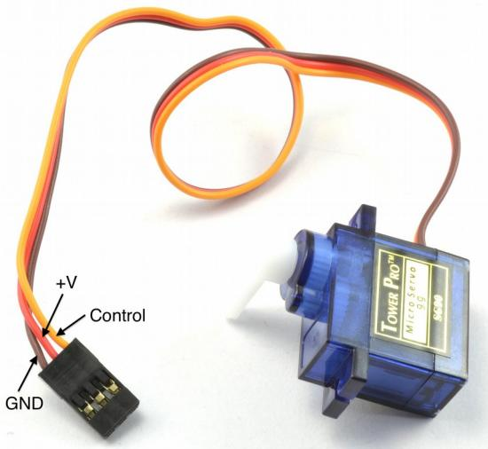
Servomotors have a 3-way connector. Two of these supply power to the servo and the third is a control signal that sets the position of the servomotor's arm. Wiring color can vary with different servomotors, but the most common are as follows:
