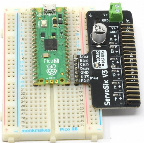
The ServoSix V3 is ideal for connecting servomotors to any breadboard-compatible microcontroller. However, it is especially suited to the Raspberry Pi Pico.
