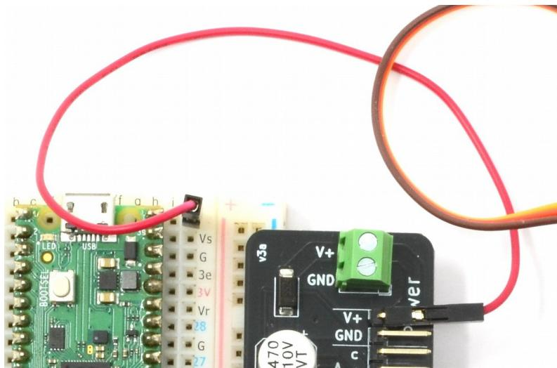
If you decide to power your servomotors from the power supply of your Pico (or other microcontroller board), you will need to connect the V+ pin (or screw terminal) of the ServoSix to the 5V supply of your microcontroller using a jumper wire. In this
