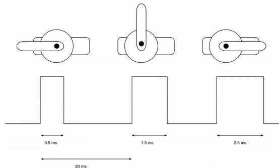
The length of each of these pulses will determine the position of the servo arm. So a short pulse of just 0.5 milliseconds will put the arm at one end of its travel. A pulse of 1.5 milliseconds will put the arm at its center position and a maximum pulse length of 2.5 milliseconds will put it at the other end of its travel.
