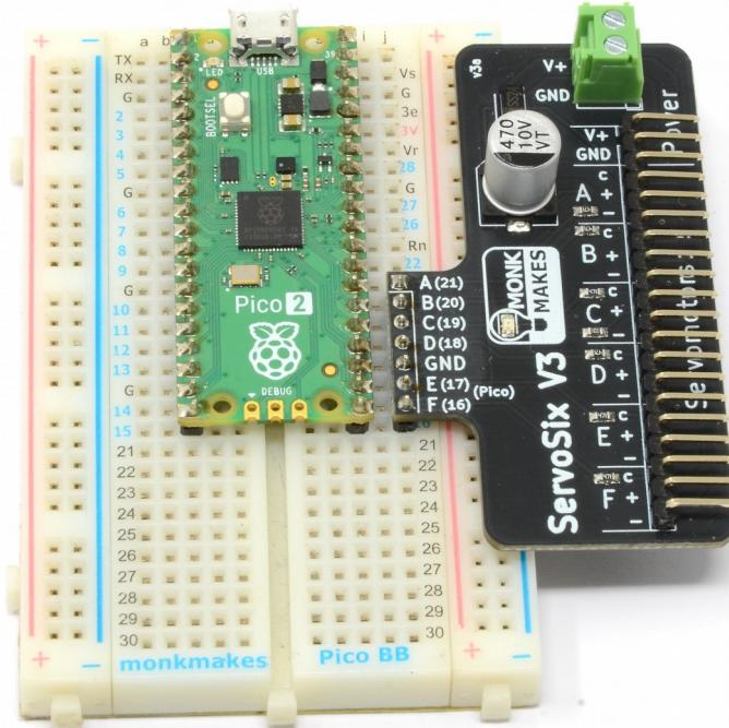
Here, a Pico 2 is fitted into a MonkMakes Breadboard for Pico which marks the pin names ([https://monkmakes.com/pico\\_bb](https://monkmakes.com/pico_bb)) making it easy to make connections to the Pico.
