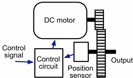
A DC motor (normal motor that can rotate continuously) is attached to a gear box, which drives the servo arm, but is also coupled to a position sensor that provides feedback to an electronic control circuit that keeps the servo arm at the correct angle.
