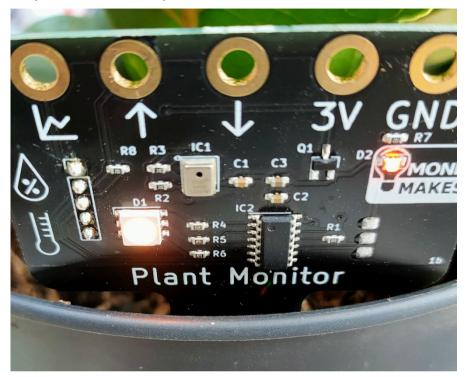
The front side of the prong should be as close to the edge of the pot as possible. The sensing all takes place from the far side of the prong.
