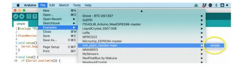
Upload the example called *Simple* to your Arduino and then open the Serial Monitor. Here, you will see a series of readings. You can also turn the Plant Monitor's LED on and off from the Serial Monitor by sending serial commands. Type L in the send area of the Serial Monitor and then press the Send button to turn the LED on, and I (lower-case L) to turn the LED off.
