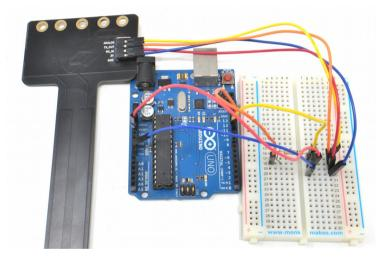
Warning: The Plant Monitor is designed to operate at 3.3V, not the 5V that some Arduinos such as the Arduino Uno operate at. So, never power the Plant Monitor with 5V and make sure that none of it's input pins receive more than 3.3V.
