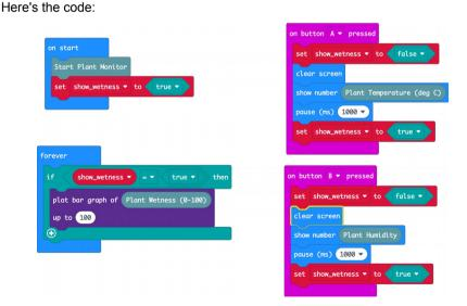
The on start block must contain the block Start Plant Monitor, that initiates communication between the micro:bit and the Plant Monitor. The variable show\_wetness is used to switch the displaying of the bar graph on and off, otherwise it will try and draw the bar graph over the top of the temperature and humidity readings.
