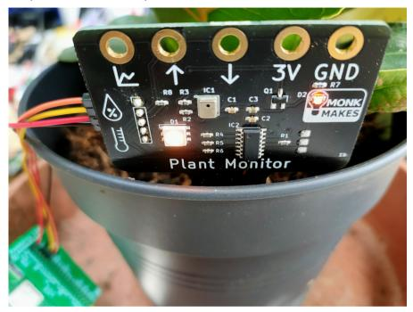
The front side of the prong should be as close to the edge of the pot as possible. The sensing all takes place from the far side of the prong.
