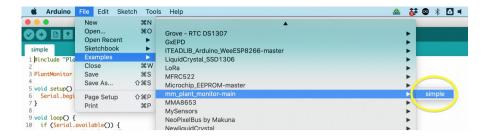
Upload the example called *Simple* to your Arduino and then open the Serial Monitor. Here, you will see a series of readings. You can also turn the Plant Monitor's LED on and off from the Serial Monitor by sending serial commands. Type L in the send area of the Serial Monitor and then press the Send button to turn the LED on, and I (lower-case L) to turn the LED off.
