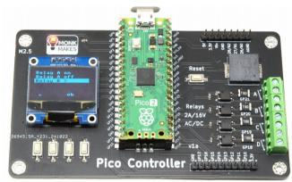
A 4-channel low-voltage Solid State Relay controller designed for the Raspberry Pi Pico. Ideal for projects involving:
