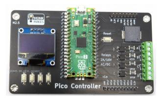
Pico GPIO (General Purpose Input Outputs) that are not used by the display, switches, relays or built-in buzzer can also be accessed using the header pins on the board, allowing sensors and other devices to be attached.
