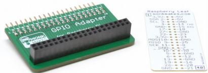
The adapter is supplied with a Raspberry Leaf GPIO template.
