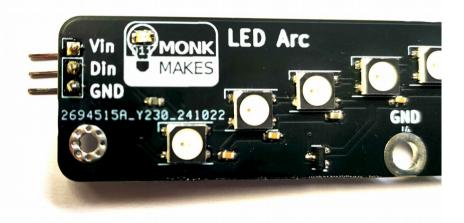
If you want to mount the LED Arc in an enclosure, and the LEDs are going to be against a front panel of some sort, then it's best to push the short end of the right-angle header pins through from the bottom of the LED Arc and solder on the top (as shown above) – as this will make it easier to attach leads.
