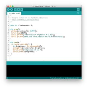
Upload the program onto your Arduino and then open the Serial Monitor. Set the baud rate to 9600 and make sure that it is set to *No line ending*.
