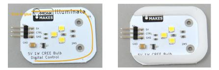
Then press the backwards-C shaped diffuser piece onto the PCB taking care not to get any glue on your fingers. Leave it to set for a couple of minutes before carrying out the next step.
