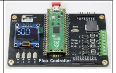
A 4-channel low-voltage Solid State Relay controller designed for the Raspberry Pi Pico.
