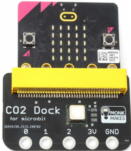
Note that the ring connectors at the bottom of the CO2 Dock are connected to the ring connectors of the micro:bit, allowing you to attach other things to your micro:bit.
