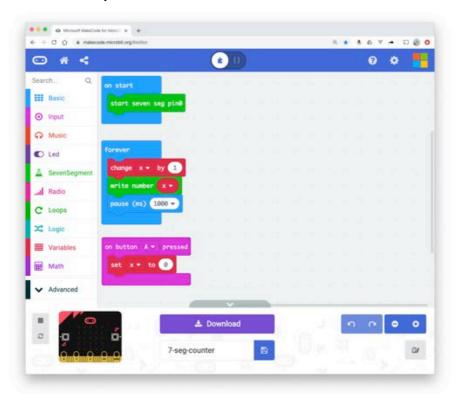
Notice how there is a new blocks category called *SevenSegment*. This is where you will find the blocks you need to use the display. The easiest way to make your own project using these blocks is to simple enter a new name for your project in the bottom center are of the window and click the save icon.
