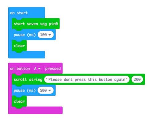
The 100 millisecond pause after the *start seven seg pin0* block is needed to give the serial port time to start working before you start sending messages. If you don't include it, you might find spurious segments display.
