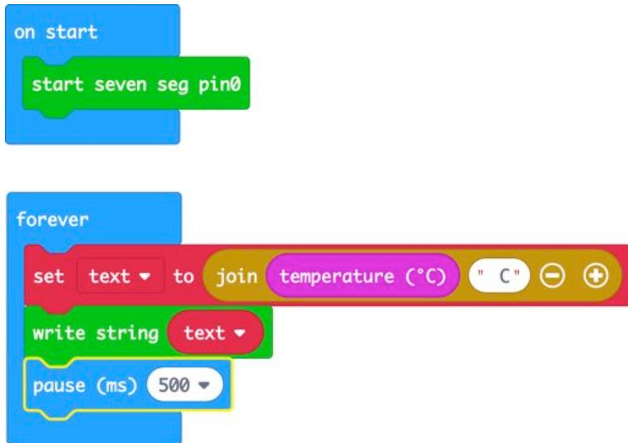
In this example, rather than using the write number block, the code constructs a string by adding a space and the C after the temperature value.
